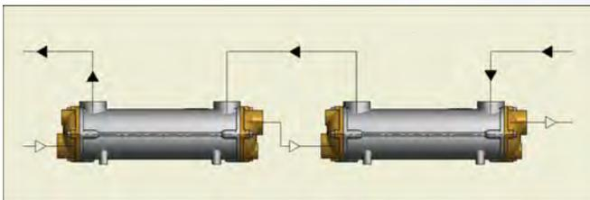
A filter with a maximum permeability of 2.0mm should be used in the water circuit of the oil cooler.
