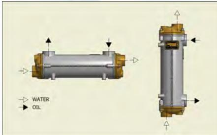
Multiple units can be connected in parallel.
