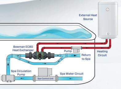
An LPG boiler system installed in each cabin provide heating for the internal room areas, plus the hot tub water. Hot water from the boiler is pumped through a Bowman EC80-5113-1T heat exchanger, which transfers the heat to the hot tub water circuit - shown in the adjacent illustration. The multi-core design of the Bowman unit is extremely efficient and with up to 25kW of heat transfer capability, can heat a commercial hot tub in around 2-3 hours from cold.
