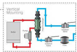
If an automatic dosing system is added, it must be installed after the heat exchanger on the return to the pool.
