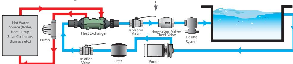
If an automatic dosing system is added, it must be installed after the heat exchanger on the return to the pool.
