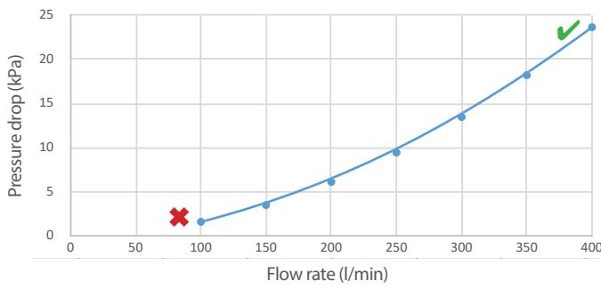
✓ Optimum heat transfer performance    ✗ Reduced heat transfer performance
