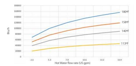
Btu/h Heat Transfer - EC100-5102-2 Pool water flow 52.8 US gpm at 82°F
