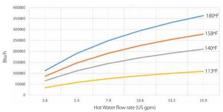
Btu/h Heat Transfer - EC160-5102-5 Pool water flow 66 US gpm at 82°F
