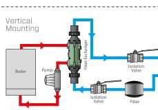
If an automatic dosing system is added, it must be installed after the heat exchanger on the return to the pool.
