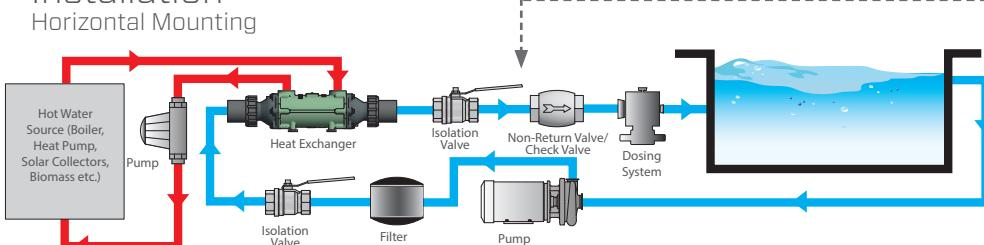
If an automatic dosing system is added, it must be installed after the heat exchanger on the return to the pool.
