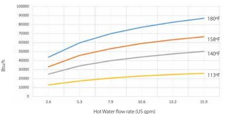
Btu/h Heat Transfer - EC80-5102-1 Pool water flow 53 US gpm at 82°F
