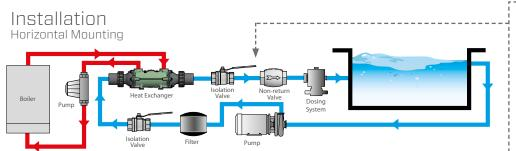
If an automatic dosing system is added, it must be installed after the heat exchanger on the return to the pool.
