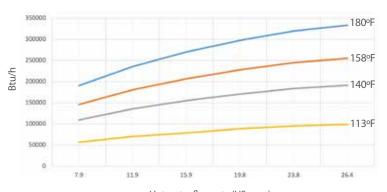
Btu/h Heat Transfer - FC100-5103-2 Pool water flow 93 US gpm at 82°F
