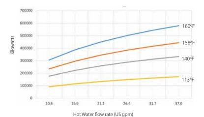
Btu/h Heat Transfer - FG100-5107-2 Pool water flow 127 US gpm at 82°F
