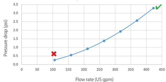
✓ Optimum heat transfer performance    ✗ Reduced heat transfer performance
