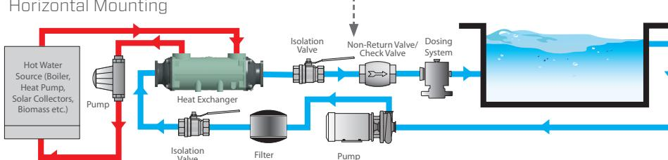
If an automatic dosing system is added, it must be installed after the heat exchanger on the return to the pool.
