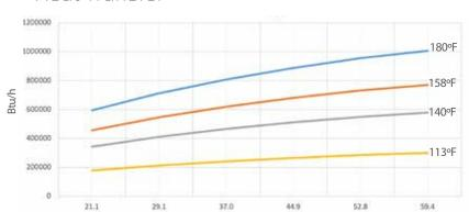
Btu/h Heat Transfer - GL140-5108-2 Pool water flow 222 US gpm at 82°F
