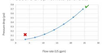
Pressure Drop Pool Water (Tube Side)
