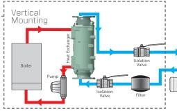
If an automatic dosing system is added, it must be installed after the heat exchanger on the return to the pool.
