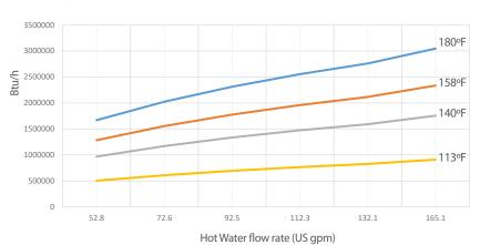
Btu/h Heat Transfer - JK190-5110-3 Pool water flow 501.9 US gpm at 82°F
